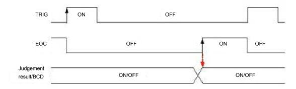
$\circ$  When the EOC signal turns on, the judgment result and BCD signals change.
