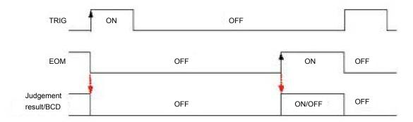
$\circ$  When the TRIG signal turns on, the judgment result and BCD signals are cleared.
